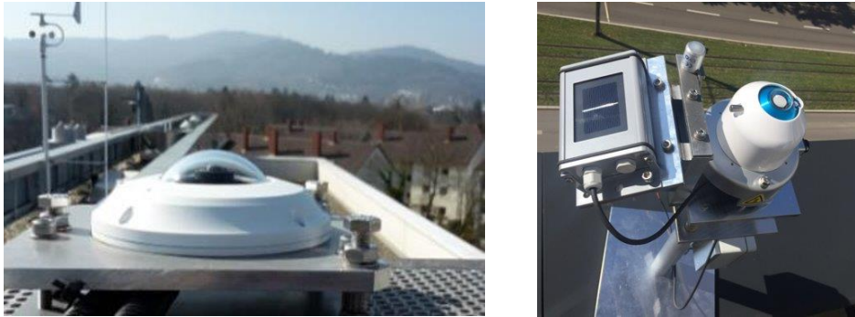
Figure 2: Fraunhofer's equipment for sky imager based solar forecasts
